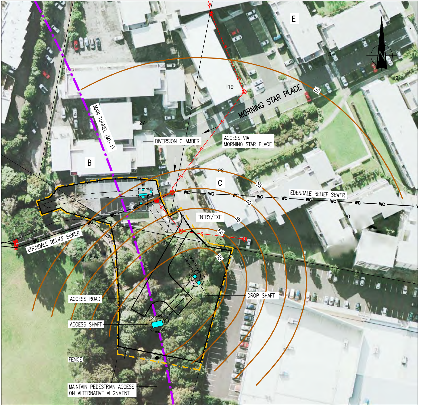
FIGURE 3 – ESTIMATED SETTLEMENT CONTOURS NOT TO SCALE PROPOSED LYON AVENUE SITE
